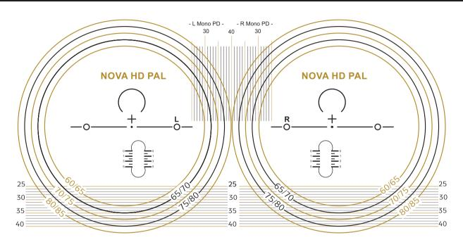
Fitting cross is located 3mm above lens Prism Reference Point
